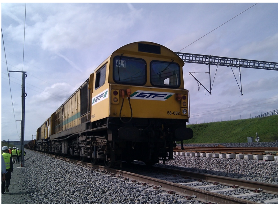
The Class 58s hired out to French infrastructure company were used on the construction of the LGV-Est, and in this view a pair are seen hauling a long welded rail train, with 58-032 at the head end, near the station that would become Belfort-Montbéliard-TGV (Meroux)
