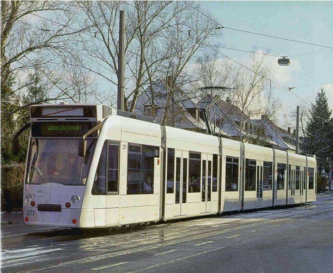
One of the new ultra low floor trams being built in 2000, with this example of the "Combino" design for Freiburg.
