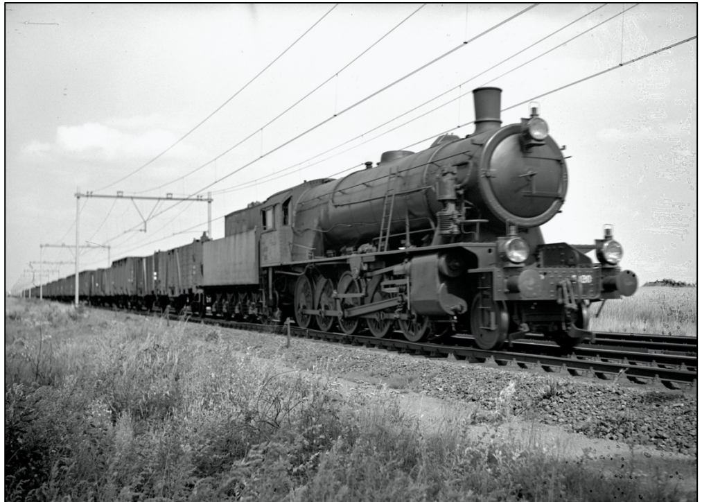
Netherlands Railways 2-10-0 No. 5020 of the N.S. series 5000/5100, with a freight train near Susteren, this locomotive was previously WD No. 73691, built by North British in 1944, and carrying Works No. 25477. Photo: 151460 / collectie Het Utrechts Archief - https://hetutrechtsarchief.nl/beeld/6E1C4CEE90CD5F91BD06D57D322CBEA0 , CCO, https://commons.wikimedia.org/w/index.php?curid=86464064
