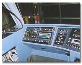
depend on the adoption and use of the "Euroradio" platform, to transmit driving authority and signal position details to the train, and in turn, details of train speed and location are passed back to the control centre.
