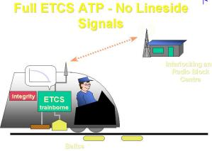
more than a set margin. TPWS has been designed to be simple to fit to existing track and trains, and unlike existing warning systems, cannot be overridden by the driver. The new ETCS platform, like previous Automatic Train Protection (ATP) systems, has two main aspects - trackside systems and the train borne equipment. Three major sub-components covering the track based equipment (Eurobalise), GSM radio communications (Euroradio) and vehicle/cab mounted equipment (Eurocab) comprise ETCS. ETCS
