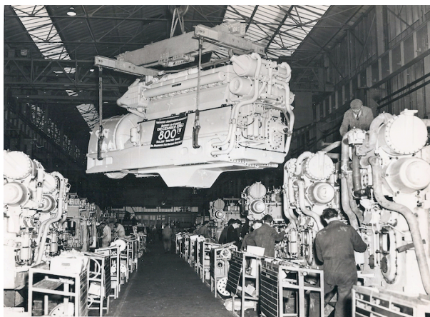
A 12 cylinder Sulzer/Vickers Christmas present for BR in December 1963 – this was the 800 th diesel from Vickers, 6LDA, 8LDA and 12LDA all built in this famous works.
