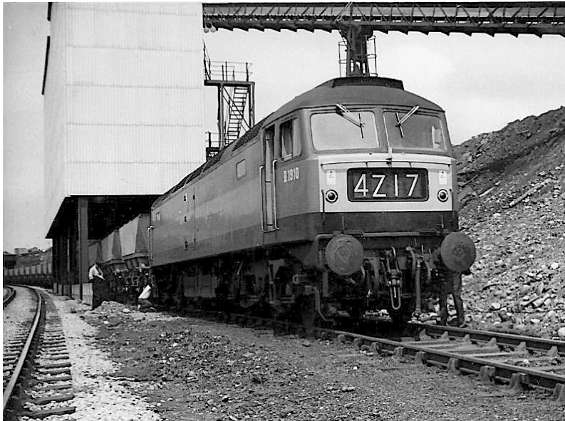
Brush Type 4 No.D1910 (later No.47 233) in BR two tone green loading coal from a hopper at the then new Blaenant Colliery with 30 new 26ton HOP AB hoppers (without the canopies which later increased their capacity to 32 tons) for Aberthaw Power Station, c.08/66.
