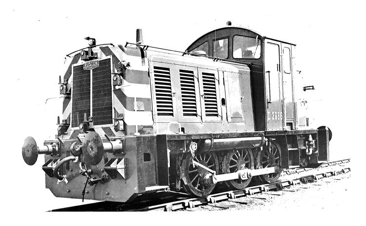
Looking like a powerful diesel shunter, these were produced by Ruston & Hornsby in 1960, and intended for use as the principal shunter for use at Southampton Docks. Later classified as '07' under the British Rail 'TOPS' scheme, they were less than successful, but certainly looked the part. © Rodger P. Bradley Collection
