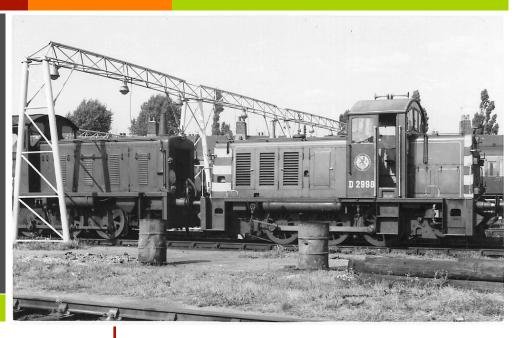
Under the 1968 classification scheme these locomotives became Class 07. In 1972 and 1973 they were renumbered as 07001-14, having previously carried numbers D2985 - D2998. Later still, a number of the class were fitted with air-brake equipment.
