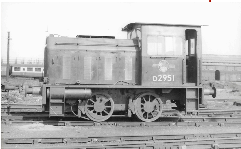
Hunslet 0-4-0 D2951 - with a distinctive small "D" prefix - was one of the three 153hp shunters ordered from the Leeds based company in 1955. Minus its final drive gearbox, flycranks and coupling rod, this example looks fairly sorry for itself. Worth noting too, is the lack of any serif to the letter D, the crest is of 1956 vintage, but the absence of hazard stripes suggest the date is between 1957 and 1961. © Lens of Sutton
