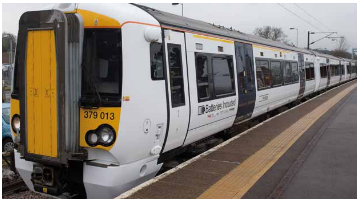
Trial conversion of a Bombardier Greater Anglia Type E Class 379 'Electrostar' EMU of 2010 to be the first IPEMU
