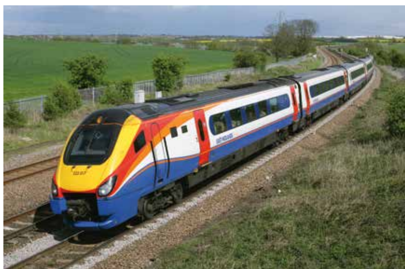
A Bombardier East Midlands Trains Type C Class 222 'Meridian' DMU introduced in 2004
