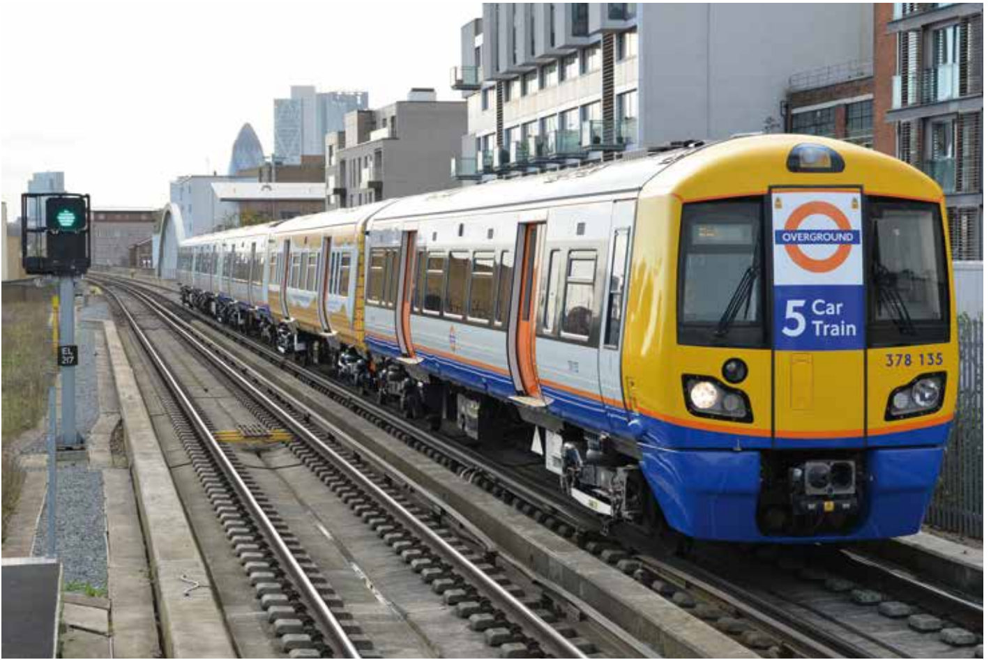
A Bombardier London Overground Type D Class 378 'Electrostar' EMU of 2008, now lengthened to 5-car formation in 2015
