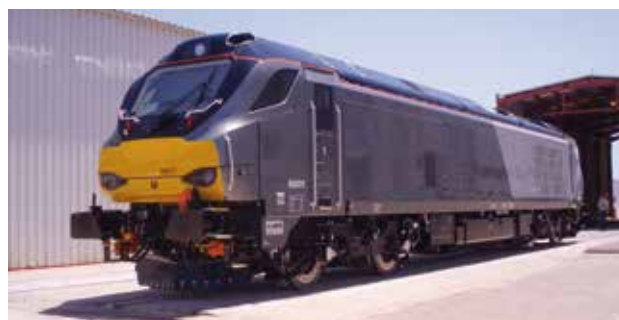
A Vossloh Type B Class 68 locomotive, being introduced on Chiltern Railways services in 2015
